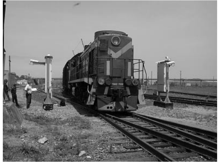
DOE’s Second Line of Defense program installs radiation detection equipment around the world at key border crossings and major shipping ports (or “megaports”) to detect the movement of nuclear or radiological materials. Budgets for the program have increased significantly since the 9/11 attacks. Source: U.S. Department of Energy
